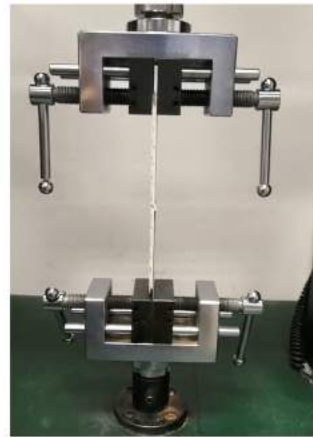
surface peeling test
